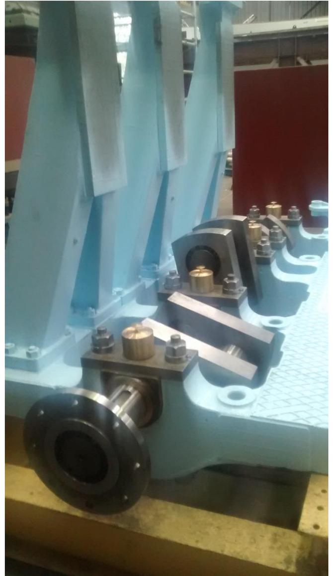
*Engine bed, new crankshaft and machined crosshead*
